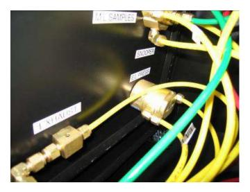
**Note:** In the event you are reconnecting a Swagelok fitting install the tubing with a hand tight, snug connection and follow up 1/4 turn with appropriate wrench. Verify connection is sealed, if not apply additional torque until connection is sealed
